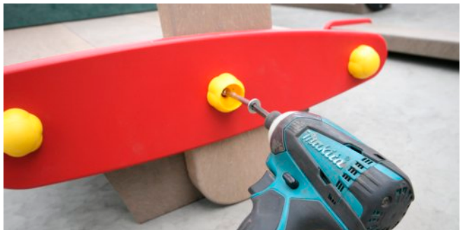
fix the wing supports by means of the two supplied screws 8 x 120 (Torx 40) and the two yellow caps
