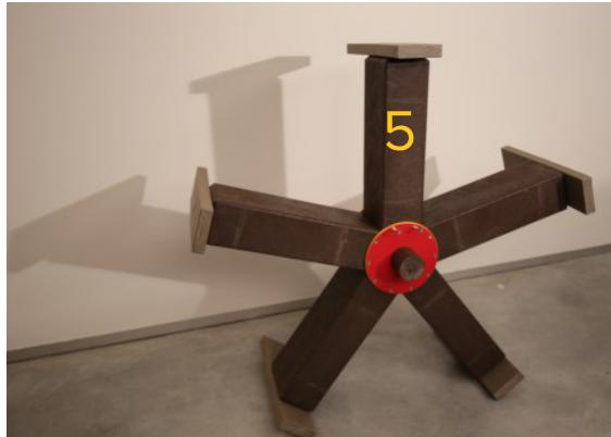
Screw the upper disc onto arm n° 5 and set upright, screw the lower disc onto arm n° 5
