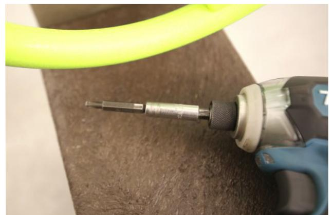
Secure the 10 steering wheels with the countersunk stainless steel screws T25 through the plastic plate. The holes in the beige boards are marked.
