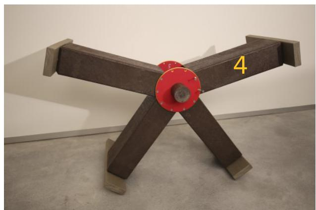
Screw the upper disc onto arm n° 4 and set upright, screw the lower disc onto arm n° 4
