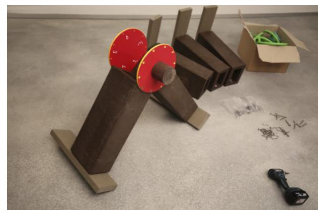
Screw the upper disc onto arm n° 2 and set this assembled part upright.
