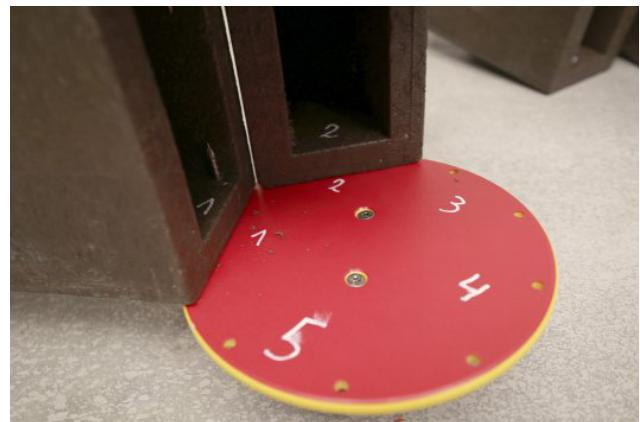
Screw the upper disc onto arm n°1 (observe the order of numbers!) and put arm n° 2 between both discs.
